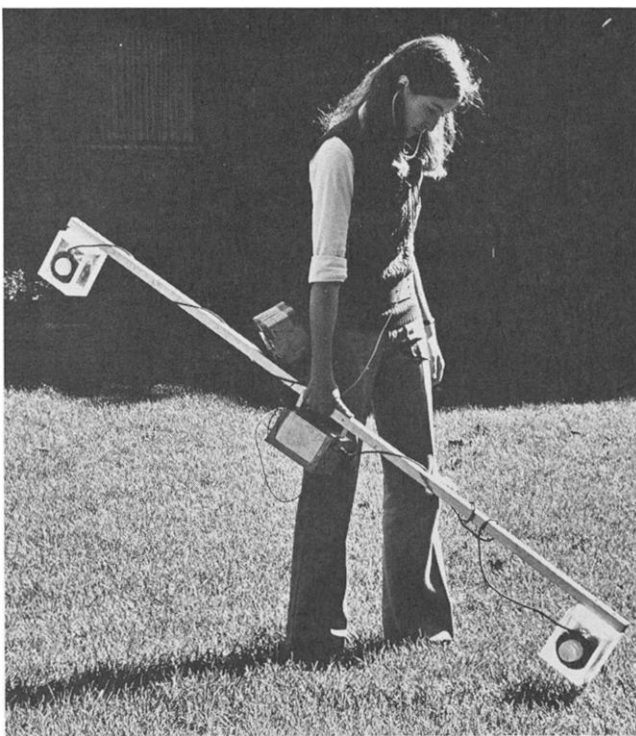
Figure 4. Operation of the portable magnetometer. Photo by Hillel Burger.
